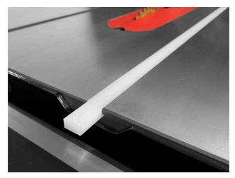
Simply place your UHMW bar into your table saw or router table miter slot to flatten and straighten the bar so you can attach the bar to your sled base. We recommend using a screw every 3" or so, although some woodworkers may space them differently.
